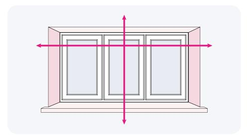
TIP: For the best results allow your blind to overlap the edges of the recess by at least 50mm on each side - ensuring that you have enough space to accommodate the suggested overlap.
