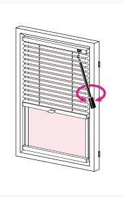
Attach the plastic wand by hooking the wand onto the tilt mechanism on the Venetian Blind.
